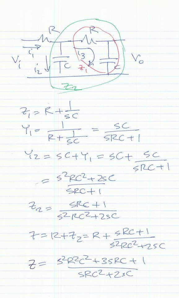
The natural response for this circuit will be given by the voots of the equation for 7, 1.e., where 7->0.  $7 = 5^{2}R^{2}C^{2} + 35RC + 1 = 0$  $5RC^{2} + 25C$  $5^2R^2C^2 + 3SRC + 1 = 0$ 5 = -3Re ± V9R2c2-4R2c2 2R2C2 For R=10x and C=0.01 uF 5, = -3,819.66 radians/sec 52 = -26,180.34 radians/see
